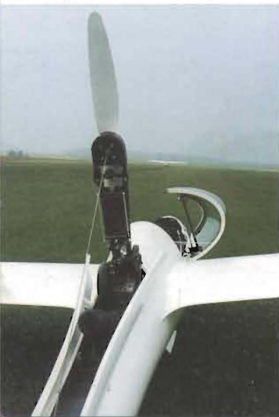
4DM propeller and buried Rotax engine.
