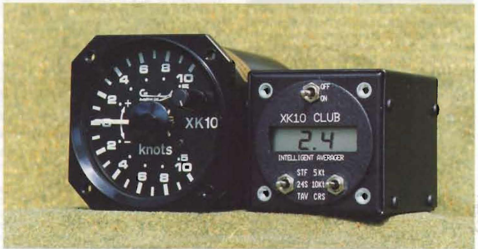
The variometer and digital averager.
